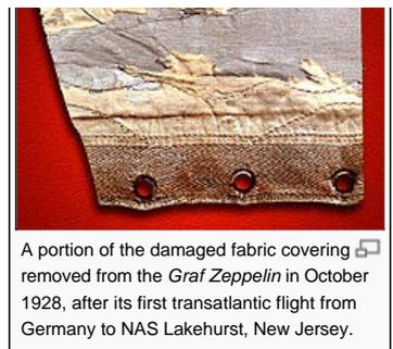
A portion of the damaged fabric covering removed from the *Graf Zeppelin* in October 1928, after its first transatlantic flight from Germany to NAS Lakehurst, New Jersey.
